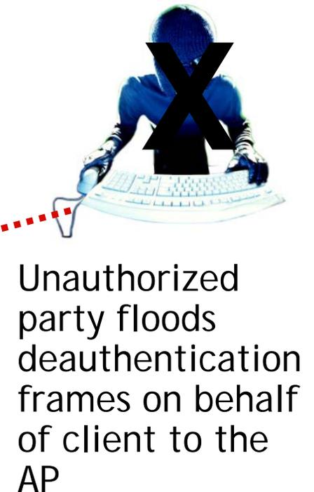
Based on location signature and client classification, the WLAN switch drops illegal deauthentication requests and generates alert
